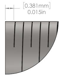
D С 4.978mm Ø0.196in OD В 4.724mm Ø0.186in ID 15F LCHT - 0.196 x 0.186 - 0.015 Pitch, 120 Cut 24 Uncut (2.5 CPR) А PART NUMBER: SIZE CONFIDENTIAL AND PROPRIETARY SY-027700 THIS DRAWING CONTAINS CONFIDENTIAL AND PROPRIETRAY В INFOMATION THAT IS THE SOLE PROPERTY OF SYMMETRY LLC. DISCLOSURE OF SAID INFORMATION DOES NOT CONSTITUTE THE RELEASE OF ANY PROPRIETARY RIGHTS THEREIN Sheet 1 of 1 DO NOT SCALE SCALE 5:1
